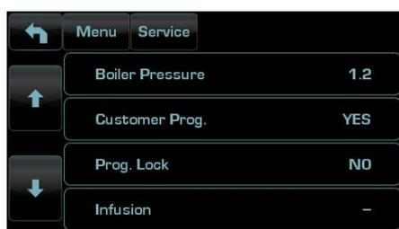
**Boiler Pressure** - indicates the pressure of the boiler; 0.6 to 1.6 bar (9 to 23 psi)
