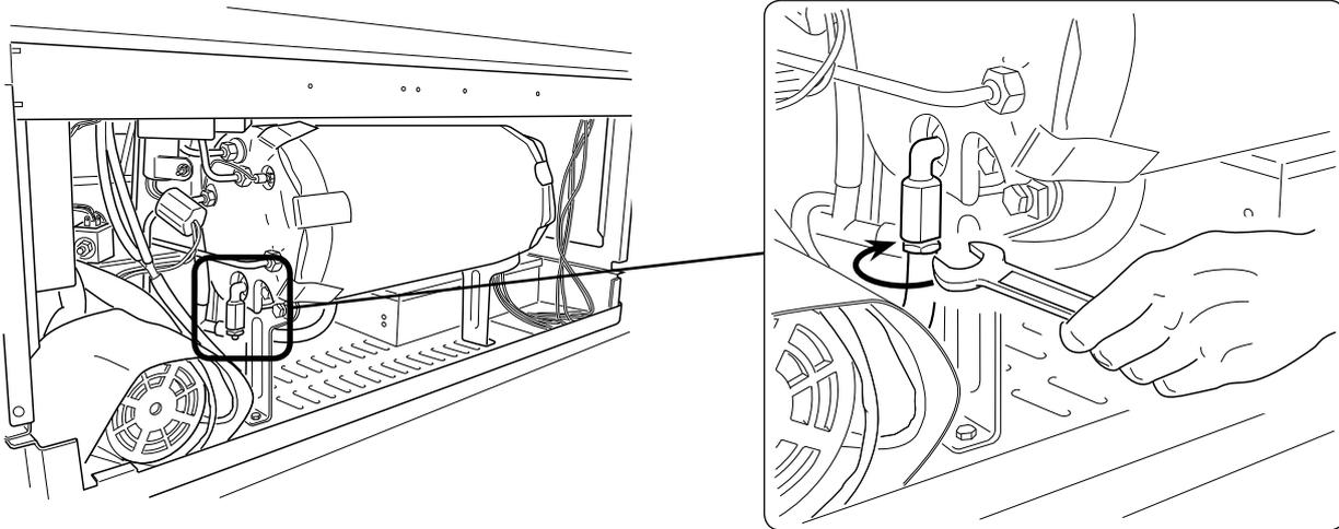
Slip a tube on the drain fitting and turn the nut in the direction indicated in the future.
