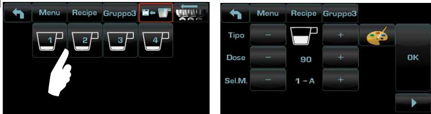
By pushing the coffee buttons on the services display, the doses entered can be viewed, with the values of the impulses of the volumetric dosing devices.
