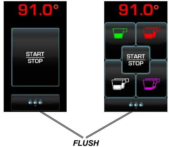
If you want to interrupt this cycle, it is possible to stop the dispensing at any time by pressing any key on the unit.
