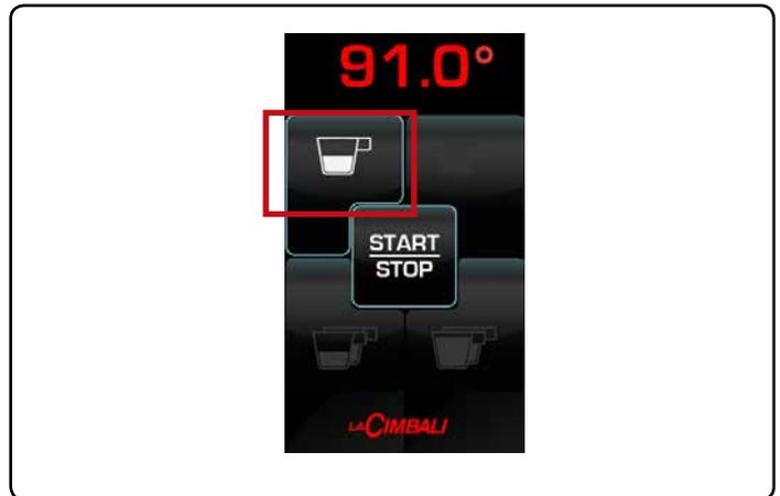
Dispensing will remain active for 2 minutes. During this time, the grinder/dispenser used will be blocked and therefore unable to grind a second dose of coffee.
