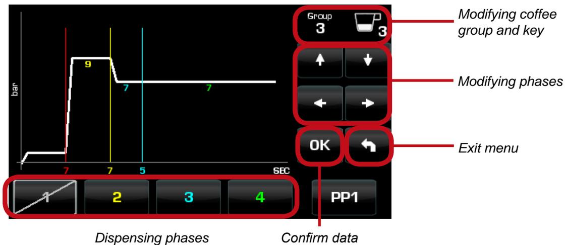
For example, **phase 2 (in yellow)** will have a duration of 7 seconds at 9 bars; **phase 3 (in blue)** will have a duration of 5 seconds at 7 bars.
