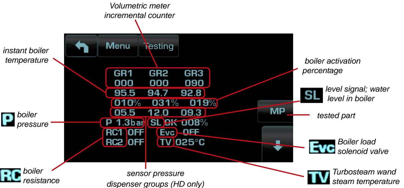
**Boiler activation percentage:** Modulation percentage of the heating power of the boiler.
