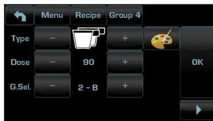
Every button on the machine can be configured based on the type and the relative grinder/dispenser. Not all types can be used with the BDS system. The possible choices are:
