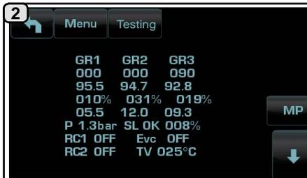
The test screen permits manual operation of the components in the machine.
