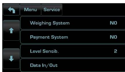
**Weighting system** - allows management of the Acaia scales for weighing the amount of coffee dispensed: YES/NO.
