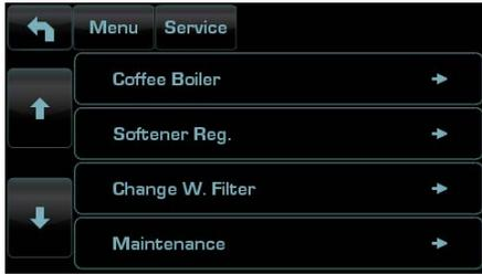
**Coffee Boiler** - this parameter includes the items for setting the coffee boiler temperature; values that can be set are 60°C to 110°C (140°F to 230°F) with steps of 0.5°C. Group temperature programming with offset correction possible (see section in pages below).
