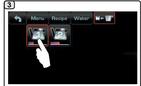
Press key to be programmed. When the desired level is reached in the container press the key again. Continue with any additional programming of the keys.
