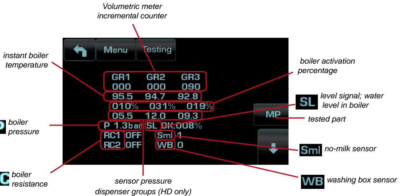
**Boiler activation percentage:** Modulation percentage of the heating power of the boiler.
