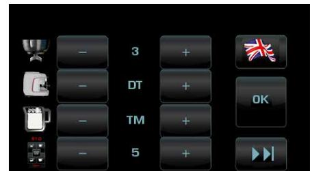
The display test procedure can be performed at any time by starting the machine with Dip 5 ON.
