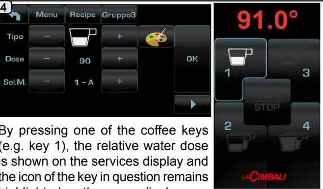
By pressing one of the coffee keys (e.g. key 1), the relative water dose is shown on the services display and the icon of the key in question remains highlighted on the group display.
